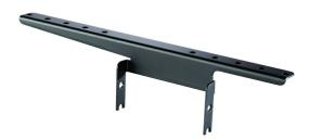
Mounts to the top side of the Mighty Mo rack channels or frames, providing mounting for runway (ladder rack) to run parallel with the row of racks. Standard brackets position the bottom of the runway at  $2^{\circ}$  above the rack height and 6" high brackets position the bottom of the runway at 6" above the rack height.
