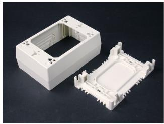
Cover snaps onto base - no screws required. Cover has twistouts on all sides. Rectangular KO in base for extenstion to wall box. Used with 2700, 2800, 2900 and NM2000 Series Raceways. 4 3/4" L x 3" W x 1 3/4" D (121mm L x 76mm W x 44mm D). 1-Gang.
