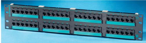
Clarity 5E 48-Port High Density Patch Panel is component compliant to EIA/TIA Category 5e performance requirements It occupies two rack units and measures 19" x 3.5". Jacks an grouped in six-port modules. Part of the Clarity 5E link and channel solution that provides significant installed performance headroom.
