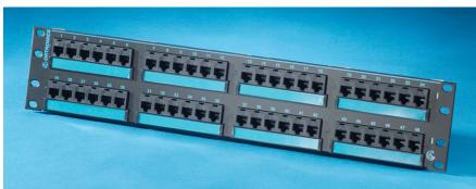
Clarity 6 48-port high density Category 6 patch panel is component compliant to EIA/TIA Category 6 performance requirements. It occupies two rack units, and measures 19" x 3.5". Jacks are grouped in six-port modules. Part of the Clarity 6 link and channel solution that provides significant installed performance headroom.
