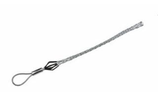
Junior Duty, Flexible Eye. Cable Diameter - 1.000-1.240-inch, Mesh Length - 12-inch, Break Strength - 4,100 lbs.
