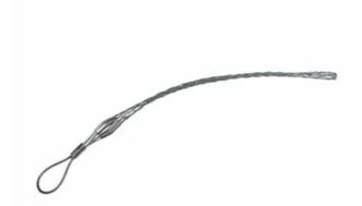
Light Duty, Standard Length, Flexible Eye. Cable Diameter - 2.000-2.490-inch, Mesh Length - 26-inch, Break Strength - 10,000 lbs.
