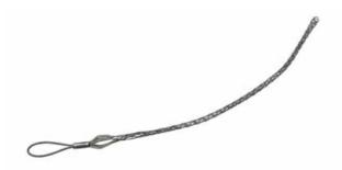
Medium duty, Flexible eye. Cable Diameter - 0.500-0.740-inch, Mesh Length - 17-inch, Break Strength - 3,400 lbs.
