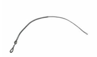
Medium-duty, Long length, Flexible eye. Cable Diameter - 0.750-0.990-inch, Mesh Length - 48-inch, Break Strength - 8,100 lbs.
