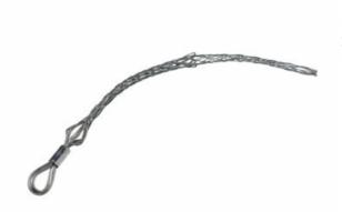
Medium Duty, Short Length, Flexible Eye, T-Type. Cable Diameter - 2.000-2.490-inch, Mesh Length - 24-inch, Eye Diameter - 7/16-inch, Break Strength - 18,500 lbs.
