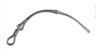
Medium Duty, Short Length, Flexible Eye, T-Type. Cable Diameter - 2.500-2.990-inch, Mesh Length - 24-inch, Eye Diameter - 1/2-inch, Break Strength - 24,500 lbs.
