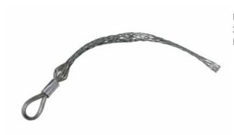
Medium Duty, Short Length, Flexible Eye, T-Type. Cable Diameter - 3.500-3.990-inch, Mesh Length - 26-inch, Eye Diameter - 5/8-inch, Break Strength - 31,000 lbs.
