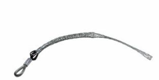
Medium Duty, Standard Length, Flexible Eye, T-Type. Cable Diameter - 3.500-3.990-inch, Mesh Length - 40-inch, Eye Diameter - 5/8-inch, 31,000 lbs.
