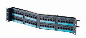
Clarity® SNAPTM patch panels offer improved rear cable management with the addition of an adjustable depth rear management bar. The rear portion of these bars is also removable to provide more working room for the initial termination of panels. After cables are SNAP terminated, the rear bars are attached and adjusted to the depth that best matches the cable and rack selections.
