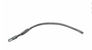
Heavy-Duty, Short Length, Rotating Eye, K-Type. Cable Diameter - 0.500-0610-inch, Mesh Length - 16-inch, Eye Diameter - 7/8-inch, Break Strength - 5,600 lbs.
