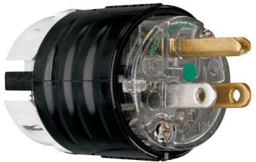
Straight Blade Hospital Grade Plug, double pole andthree wire, unit arrives completely ready-to-wire, cutting installation time significantly. Its nylon housing provides impact and chemical resistance. Its rugged two-piece cord grip provides more uniform cord retention and the internal dust shield keeps terminals free of contaminants. 15amp 125volt.
