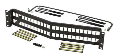
48 port unloaded angled panel for rear loading HDJ series of jacks and accessories. Includes rear management bar and straps. Occupies 2 rack units of space, 3.5" x 19".
