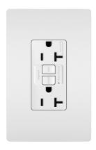
PlugTail® Spec-Grade Tamper-Resistant 20A Self-Test Duplex GFCI. Self-test GFCI Technology - conducts an automatic test every three seconds, ensuring it's always ready to protect. PlugTail® devices and connectors mean that device installation is the same regardless of skill level of the installer. The UL-Listed connectors are keyed to ensure proper wiring installation into each receptacle.
