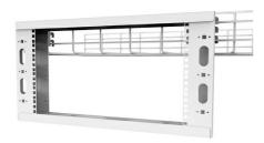
Overhead rack to support additional rack space above existing racks or cabinets. Easily installs to wire cable tray, tubular runway, or threaded rod. The racks are fully assembled and bonded as packaged. The racks are available in 2RU thru 8RU, in black or white to match any installation. Used when floor space is at a premium or for easy top of rack cable patching.
