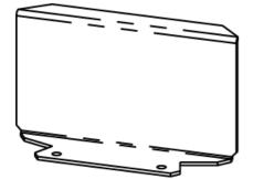
Used to close off unused gangs. NOTE: For use with RFB4E, RFB6 and RFB6E Series Floor Boxes.
