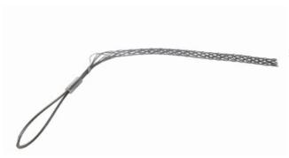
Double Weave, Standard Length, Closed Mesh, Offset Eye. Cable Diameter - 1.250-1.490, Mesh Length - 17-inch, Break Strength-5,500 lbs.
