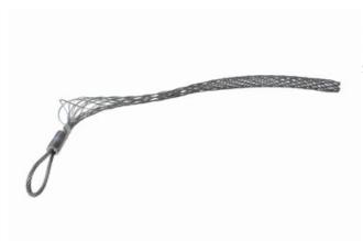
Double Weave, Long Length, Closed Mesh, Offset Eye. Cable Diameter - 2.500-2.990-inch, Mesh Length - 30-inch, Break Strength- 11,000 lbs.
