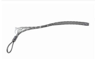
Double Weave, Long Length, Closed Mesh, Offset Eye. Cable Diameter - 3.000-3.490-inch, Mesh Length - 33-inch, Break Strength - 16,000 lbs.
