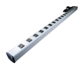
Sixteen outlets, rugged gray aluminum housing, 15A, 15' (4.6m) 14/3 SJT black cord with NEMA5-15 plug. Length 48" (1.2m). Receptacle center-to-center 2 1/2" (64mm). Snap-on, slide-off mounting.
