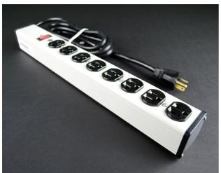
Eight 20A, 120V, 60Hz, 2500 watt outlets, lighted switch, putty white aluminum housing, 15' [4.6m] 12/3 SJT black cord with NEMA5-20 plug. Length 17 1/4" [438mm]. Receptacle center-to-center 1 1/2" [38mm]. Snap-on slide-off mounting.
