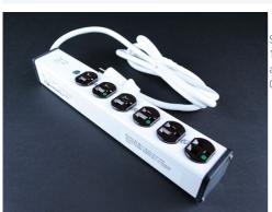
Six outlets. Rugged white aluminum housing. 15' (4.6m) 14/3 SJT white cord with NEMA5-15 plug. Length 13 1/4'' (337mm). Receptacle center-to-center 1 1/2'' (38mm). Snap-on, slide-off mounting. cTUVus Listed as Medical Electrical Equipment. NOTE: Suitable for use where Article 517 of NEC requires Hospital Grade Outlets.
