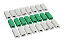
W30 - For common connection of two, three or four No. 12 or No. 14 solid copper conductors. Packed 24 pieces per carton (16 W30 and 8 W30G). W30G - For connection of equipment grounding of 2, 3, or 4 solid conductors No. 14 or No. 12 AWG. 300V maximum. 20A 105 degrees C maximum. NOTE: Not for use with aluminum conductors.
