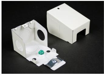
1/2" trade size KOs located on end, sides, and bottom of fitting. 3/4" KOs on bottom and rear. Includes ground screw.
