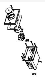
Includes single-gang box, one 15A tamper-resistant receptacle, and brass cover with one screw plug. For hole cut dimensions, see installation instructions sheet. Box Dimensions: 2 1/8" W x 3 3/4" L x 3 7/8" D (54mm W x 95mm L x 98mm D) Device Plate: 3 1/8" W x 4 15/16" L (79mm W x 125mm L).
