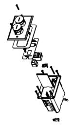
Includes single-gang box, divider, one 15A, 125V receptacle, one opening for communication device, and brass cover with two screw plugs. For hole cut dimensions, see installation instructions sheet. Box Dimensions: 2 1/8'' W x 3 3/4'' L x 3 7/8'' D (54mm W x 95mm L x 98mm D) Device Plate: 3 1/8'' W x 4 15/16'' L (79mm W x 125mm L).
