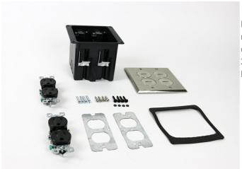
Includes dual-gang box, two 15A tamper-resistant duplex receptacles, and nickel cover with four screw plugs. For hole cut dimensions, see installation instructions sheet. Box Dimensions:  $3\ 1/4''\ W\ x\ 3\ 3/4''\ L\ x\ 3\ 7/8''\ D\ (83mm\ W\ x\ 95mm\ L\ x\ 98mm\ D)$  Device Plate:  $4\ 7/8''\ W\ x\ 5\ 1/16''\ L(124mm\ W\ x\ 129mm\ L)$ .
